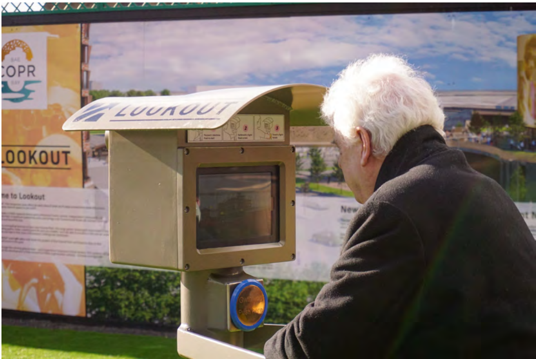
Figure 8.3: A user moving the elbow levers to pan the content of the screen.
