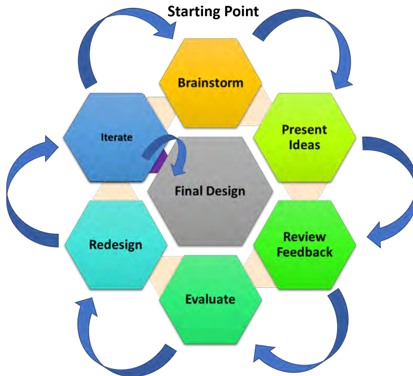
Figure 3.1: Diagram showing the methodology followed to prototype a cocreationally designed prototype. The process begins with brainstorming and travels clockwise for five iterations where a final design was confirmed.
