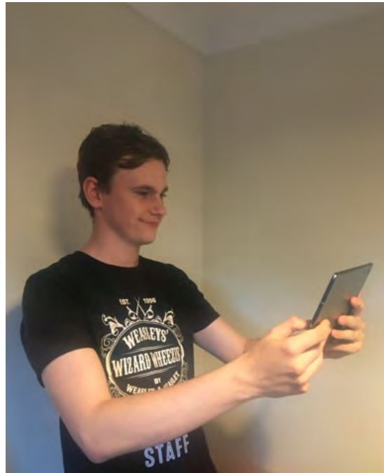
Figure 7.2: A user interacting with the final prototype and causing rotational change along the z axis of the tablet to achieve panning of the content on screen.
