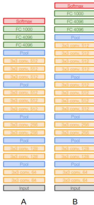
Figure 2.9: A is the 16 layer variant of the VGG Network while B is the 19 layer variant [43, 44]. All convolutional layers have 3x3 kernels with a stride of 1 and a padding of 1. All pooling layers use max-pooling and have a kernel of 2x2 and a stride of 2.
